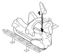
Figure 53 - Installing Log No. 4
